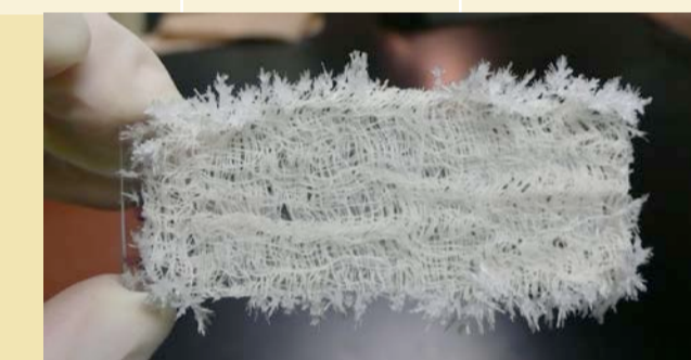
Figure 3: CDD dendrites from the 63:35 mixture.
