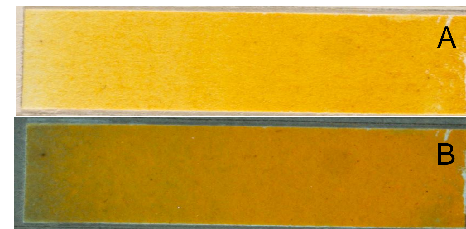
Figure 3. Photographs of a watercolour pigment book under normal (a) and UVA (b) illumination illustrating the fluorescence characteristics.
