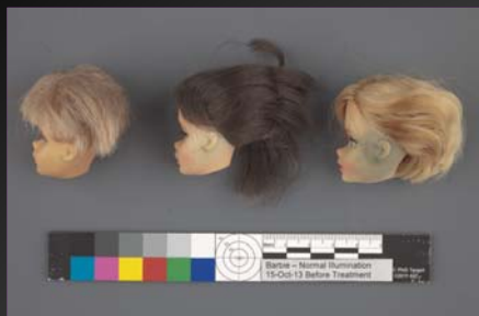
The Barbie™ head on the right has extreme "green ear syndrome" from wearing metal earrings. Below, UVC induced illumination displays the area and penetration of the stain
