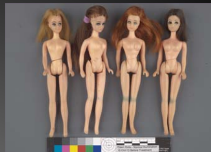
Dawn™ dolls with green staining at the knees. The dolls have articulated legs with copper alloy metal joints, seen below in x-radiograph.
