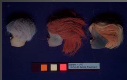
The Barbie™ head on the right has extreme "green ear syndrome" from wearing metal earrings. Below, UVC induced illumination displays the area and penetration of the stain
