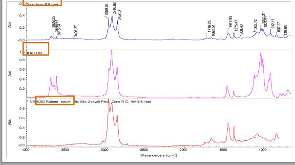
Above left: Rubber pulling away from original skin Above right: ATR-FTIR spectra comparing specimen sample, natural rubber, kaolin.
