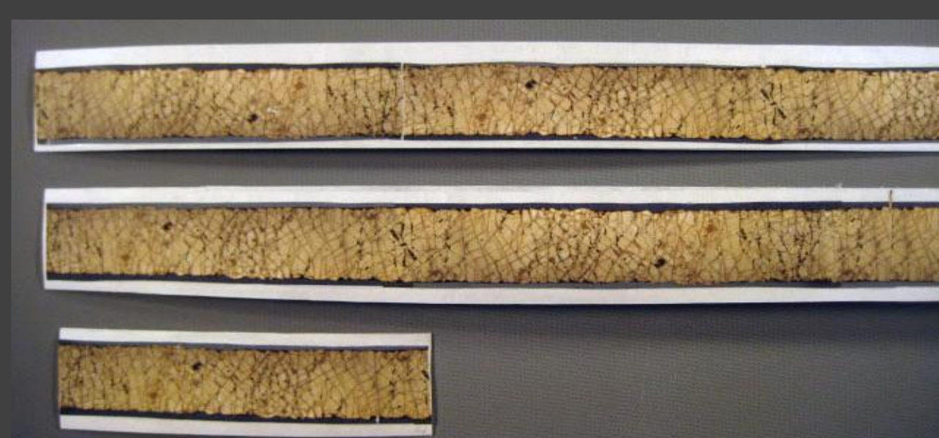
Fig. 4: Thinned printed image adhered to Tyvek backing.
