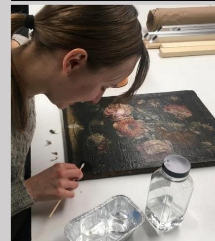
Fig. 13: Aqueous cleaning with 2% triammonium citrate in deionized water.
