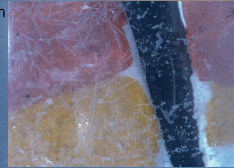
CDD crystal formation on plaster mockups
