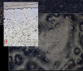
Sample M, cross-section, glaze thickness is ~200 μm (left), surface (right).
