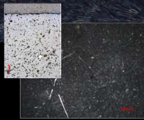
Sample T, cross-section, glaze thickness is ~100 μm (left), surface (right).
