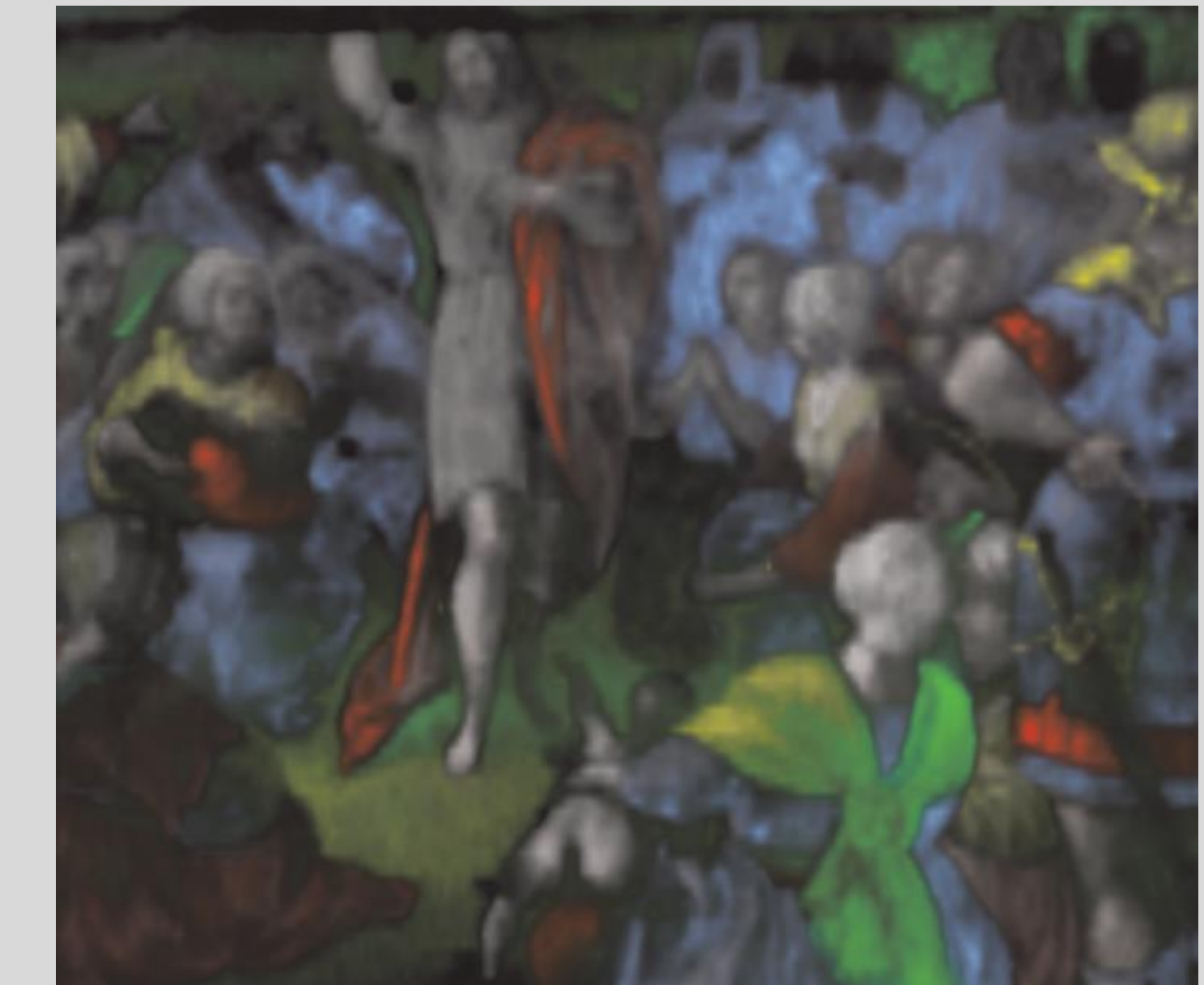
XRF false color map of five elements detected: Cu, Sn, Hg, Co, Pb (White)
