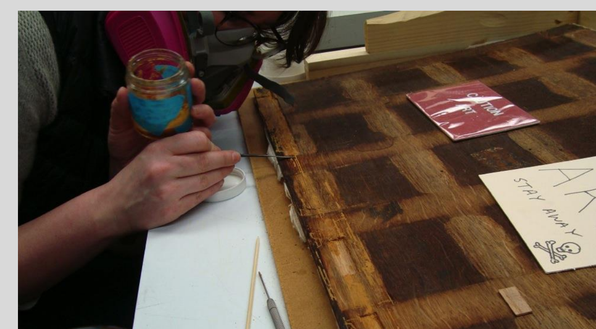
Applying the B-72 and microballoon putty
