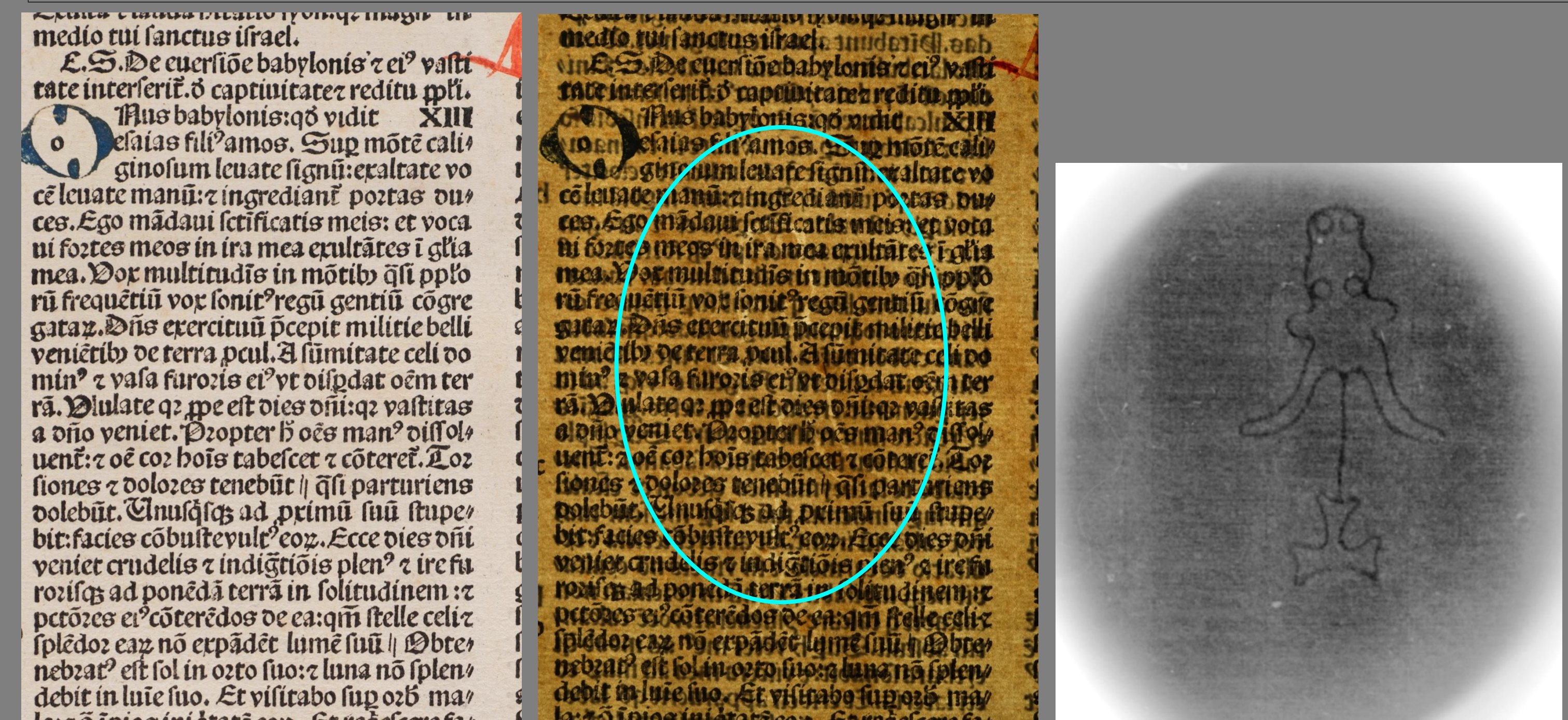
Figure 5: An 11-cm section of a written document containing watermark. Left, visible light; middle: transmitted light; right: radiograph. The circled area is where the watermark is and not discernible with transmitted light.
