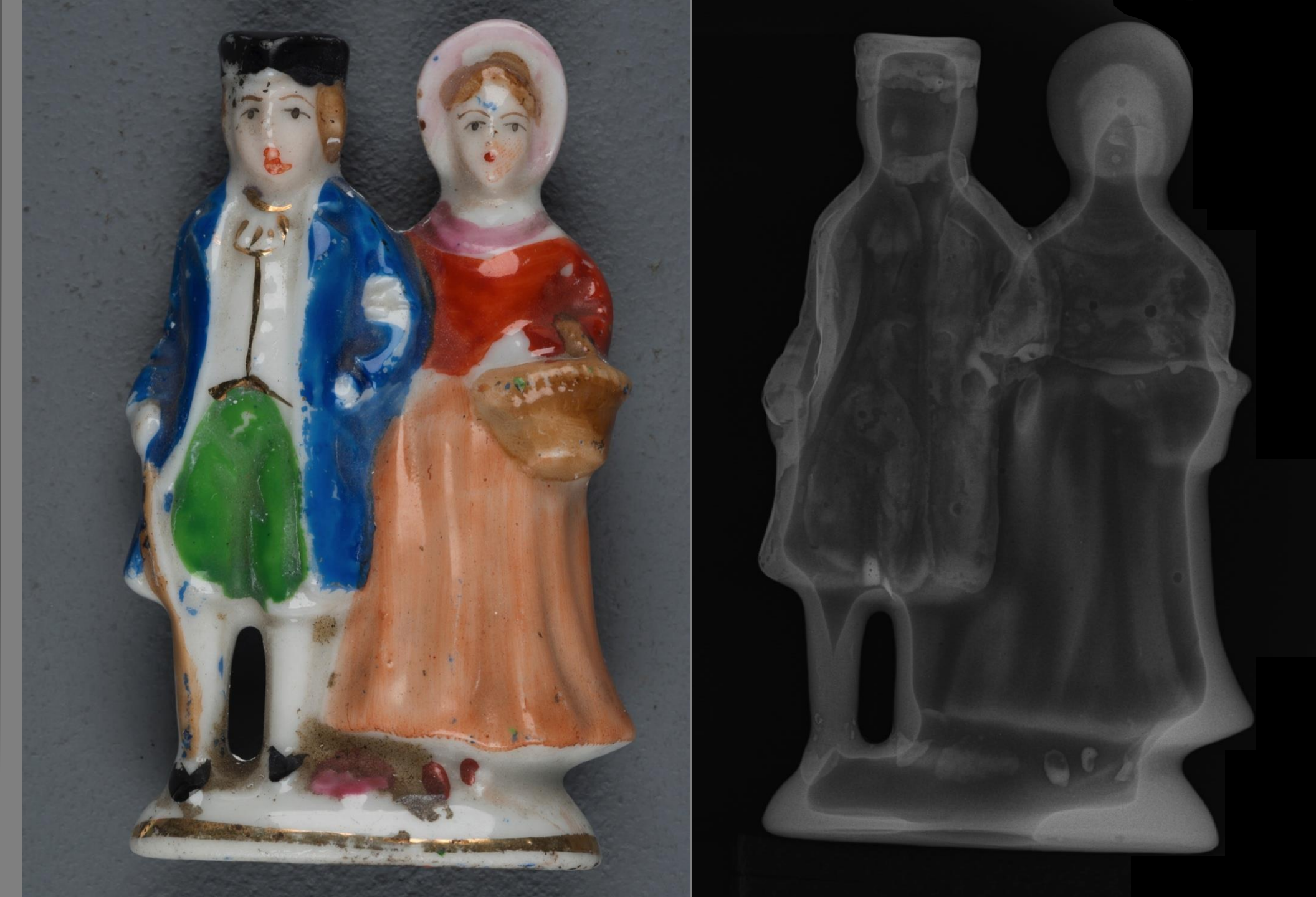
Figure 4: miniature porcelain, 7 cm high; far left: visible light; left: radiograph.
