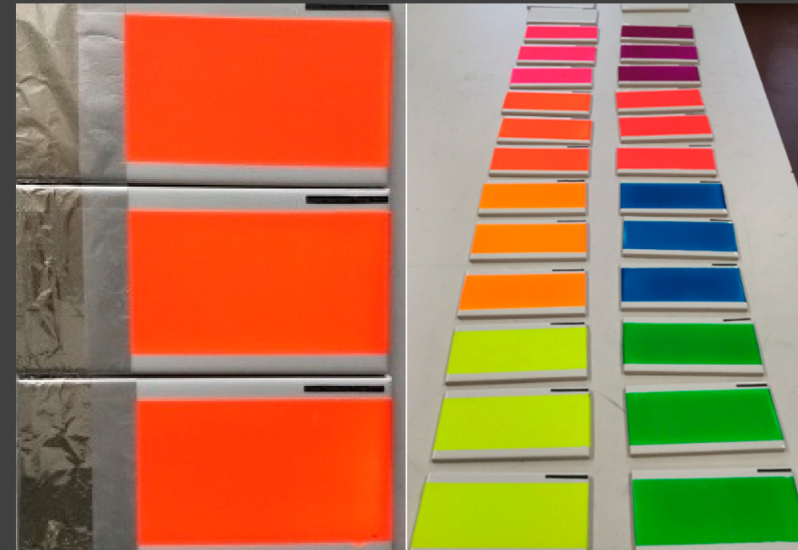
Figure 2: Sample preparation of the Kremer Fluorescent Orange (left) and all nine pigments (right) in Golden Acrylic Matte Medium prepared on white ceramic tiles.
