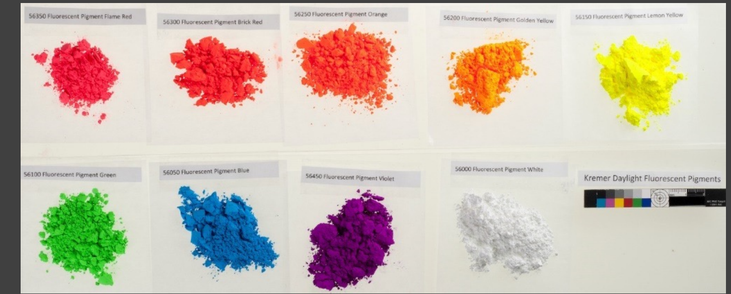
Figure 3: Kremer fluorescent pigments in powder form, as imaged in normal illumination against a whitebox.
